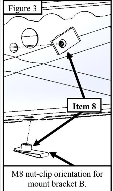
3. Take the mounting brackets and install the bracket and associated hardware loosely to its corresponding positions. For gas model bracket locations see **Figures 4 and 5**. For hardware assembly see **Figures 6 and 7**. *Do not fully tighten hardware at this time.* **Note:** On 1500 crew cab models, front positions will have a welded nut on pinch weld and must refer to **Figure 5** for bracket installation. **Note:** Bracket location is critical.
